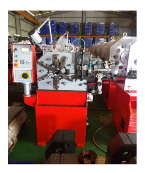
in Amax machines the motor is positioned in the top of machine, so it doesn't require such a large transmission mechanism to send power from motor to the moving mechanisms.
