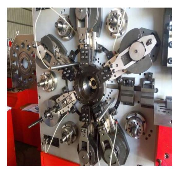
Forming axis in our machines has a bigger diameter and is stronger, stroke is longer, when producing certain parts it is visible.
