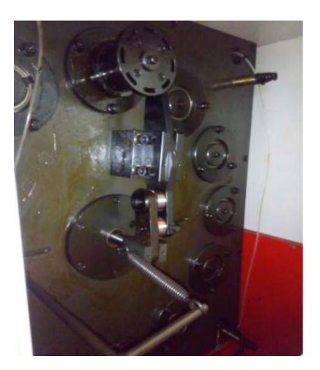
AMAX rear action slide is pushed and drawn by cams so the structure ensures the slide can be drawn in time to keep it from tool crash
