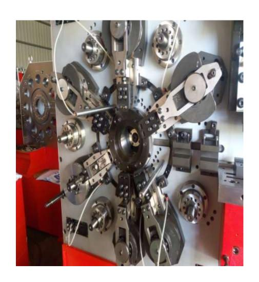
Slides of our machine equipped with dual CAMs, which guarantees long life of inner mechanism.
